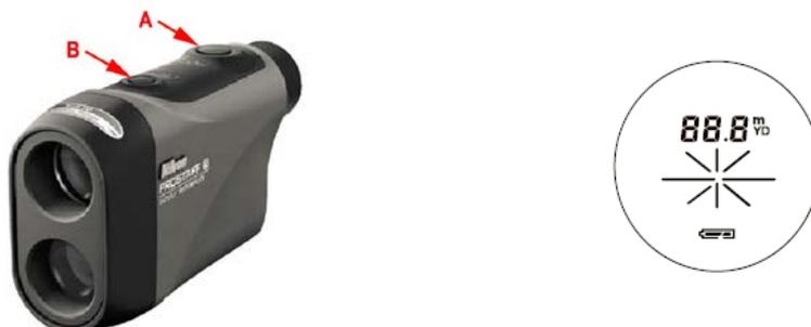
To take a measurement press the Power button **A** and the LCD illuminates, align the reticle on the target and press and hold the Power button again until the display appears as it does in the picture, right side above. To obtain the best results try to select bright colored targets with large, shiny, highly reflective surfaces.
