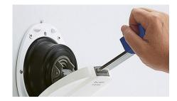
**BILGE PUMP** OSR reference 3.23 / 3.23.1 b) Bilge pump, manual, permanently installed, operable with all cockpit seats. Removable bilge pumps handle retained by lanyard.
